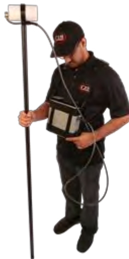
Figure 3: GSM-19T Proton Precession system in action.
