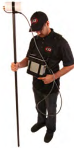
Figure 4: GSM-19T Proton Precession system in action.
