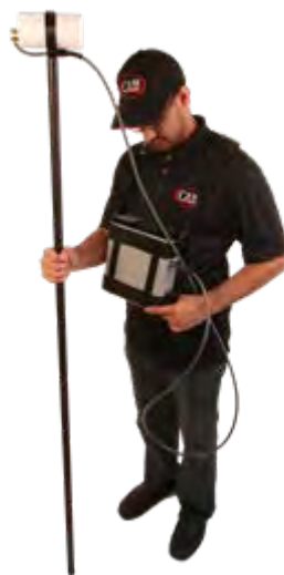
Figure 6: GSM-19T Proton Precession system in action.
