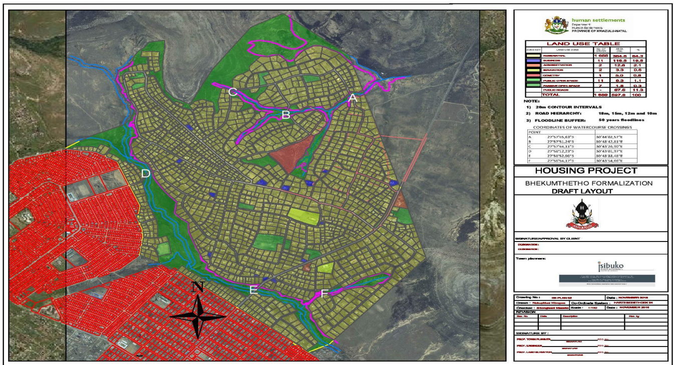
Figure 7 Site layout with sensitive areas that may be impacted (work across watercourses).
