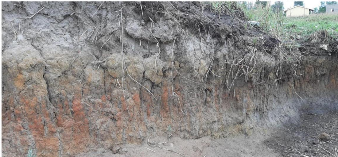
Photo 9: View of the gully side wall within the upper section of Wetland Unit S1-A. Note the grey colour of the soil and iron minerals (brown stains) that have been leached out of the soil indicating the presence of anaerobic conditions typical of wetland habitats.
