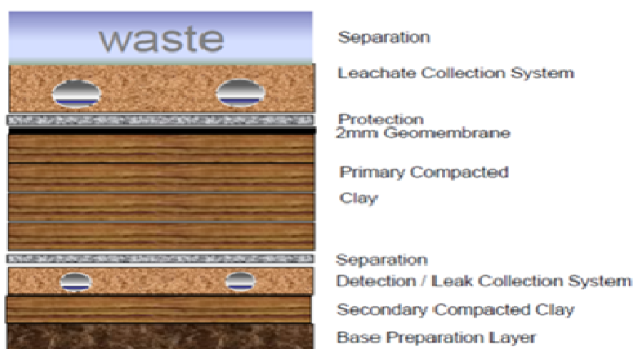
Figure 2: The different lining layers of the construction of the coal stock yard.
