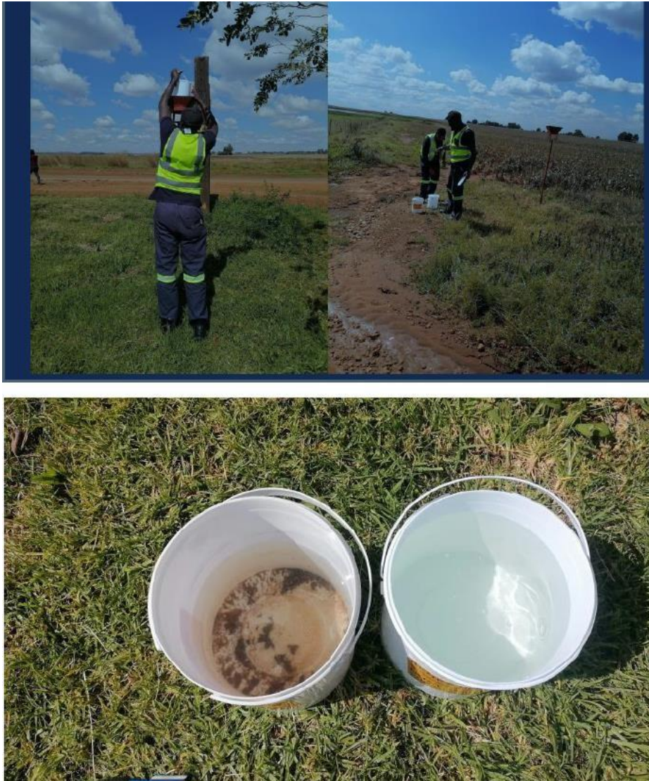
Figure 39: Dust monitoring stations (Singo Consulting(Pty)Ltd, 2023)
