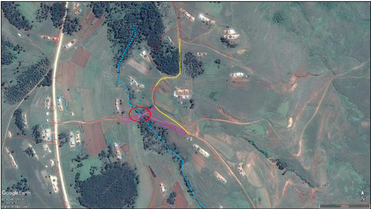
Figure 2: Example of where a river crossing was avoided (purple lines show removed pipeline) by rerouting the pipeline along an existing road (yellow line; source: Google Earth Pro, 2017).
