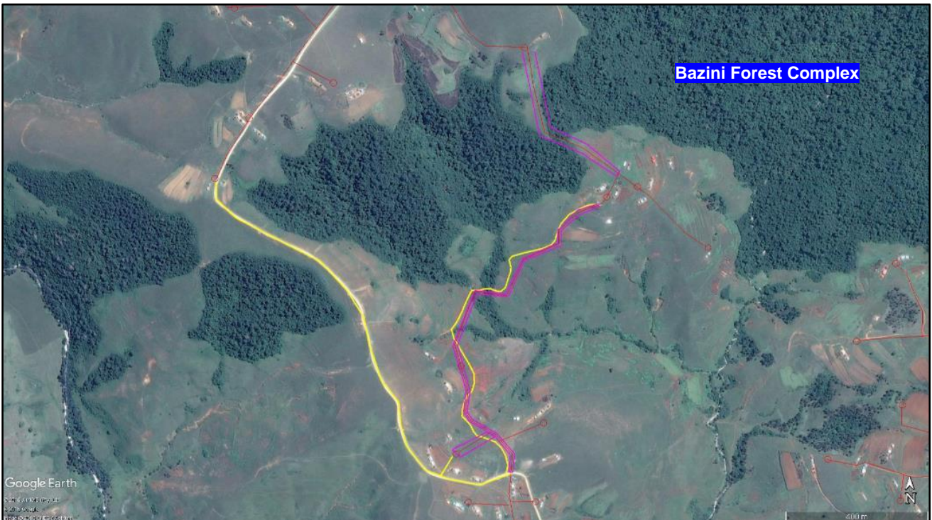
Figure 4: The original pipeline route through the Bazini forest was rerouted to avoid traversing through the forest and to provide a greater buffer zone between the forest edge and the pipeline. Layout Alternative 2, now follows existing roads and foot paths to reduce the impact on the Bazini forest (yellow line; source: Google Earth Pro, 2017).
