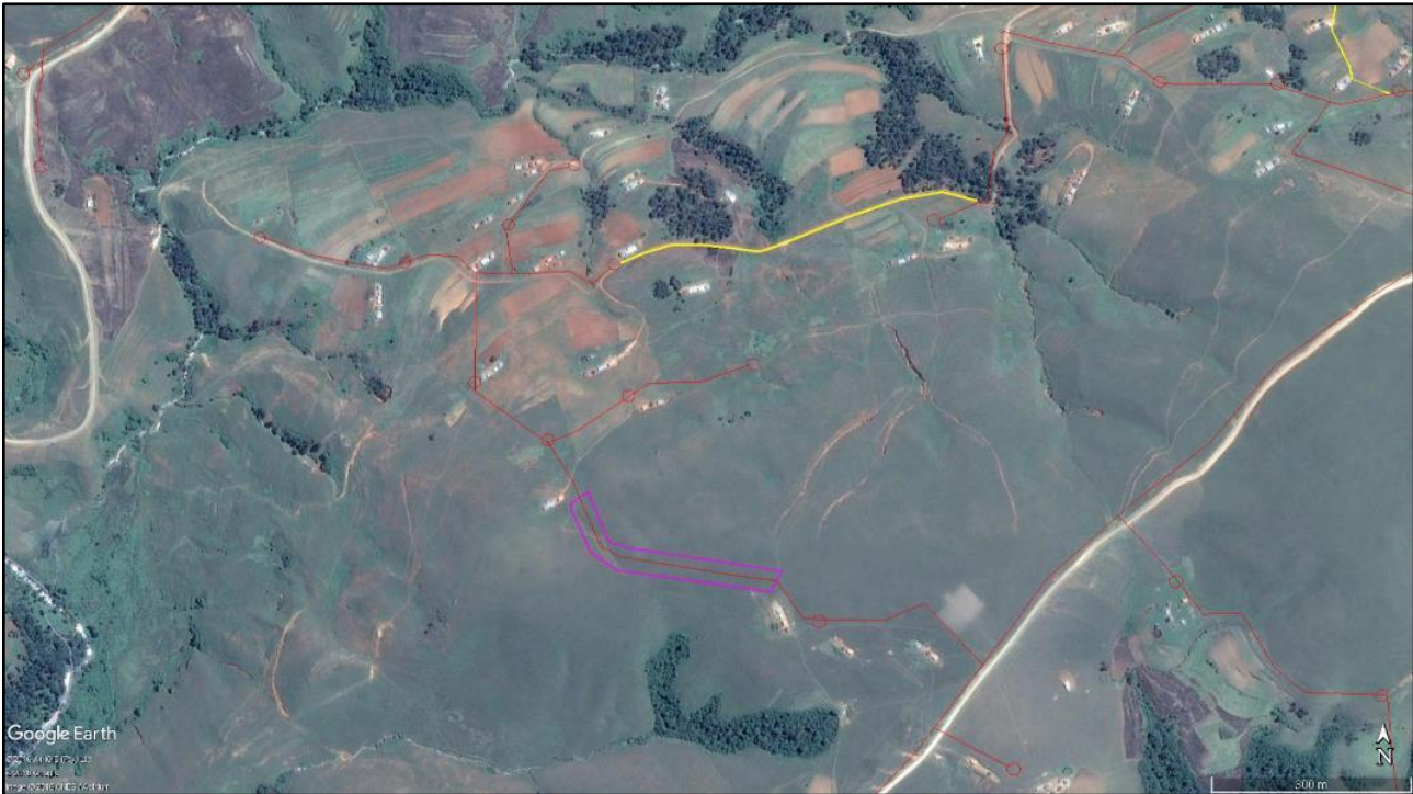
Figure 5: Original pipeline route traversing a steep sloop was avoided (purple lines show removed pipeline; source: Google Earth Pro, 2017).
