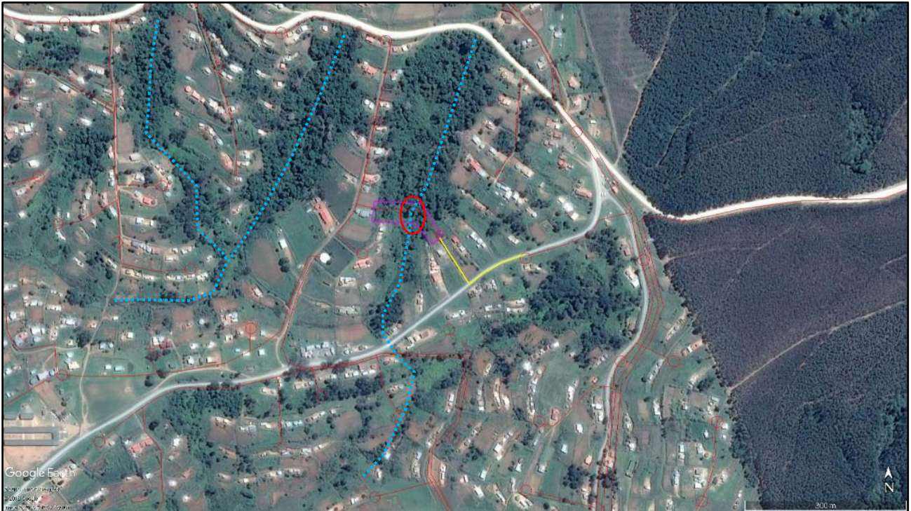
Figure 4: The original pipeline route through the Bazini forest was rerouted to avoid traversing through the forest and to provide a greater buffer zone between the forest edge and the pipeline. Layout Alternative 2, now follows existing roads and foot paths to reduce the impact on the Bazini forest (yellow line; source: Google Earth Pro, 2017).
