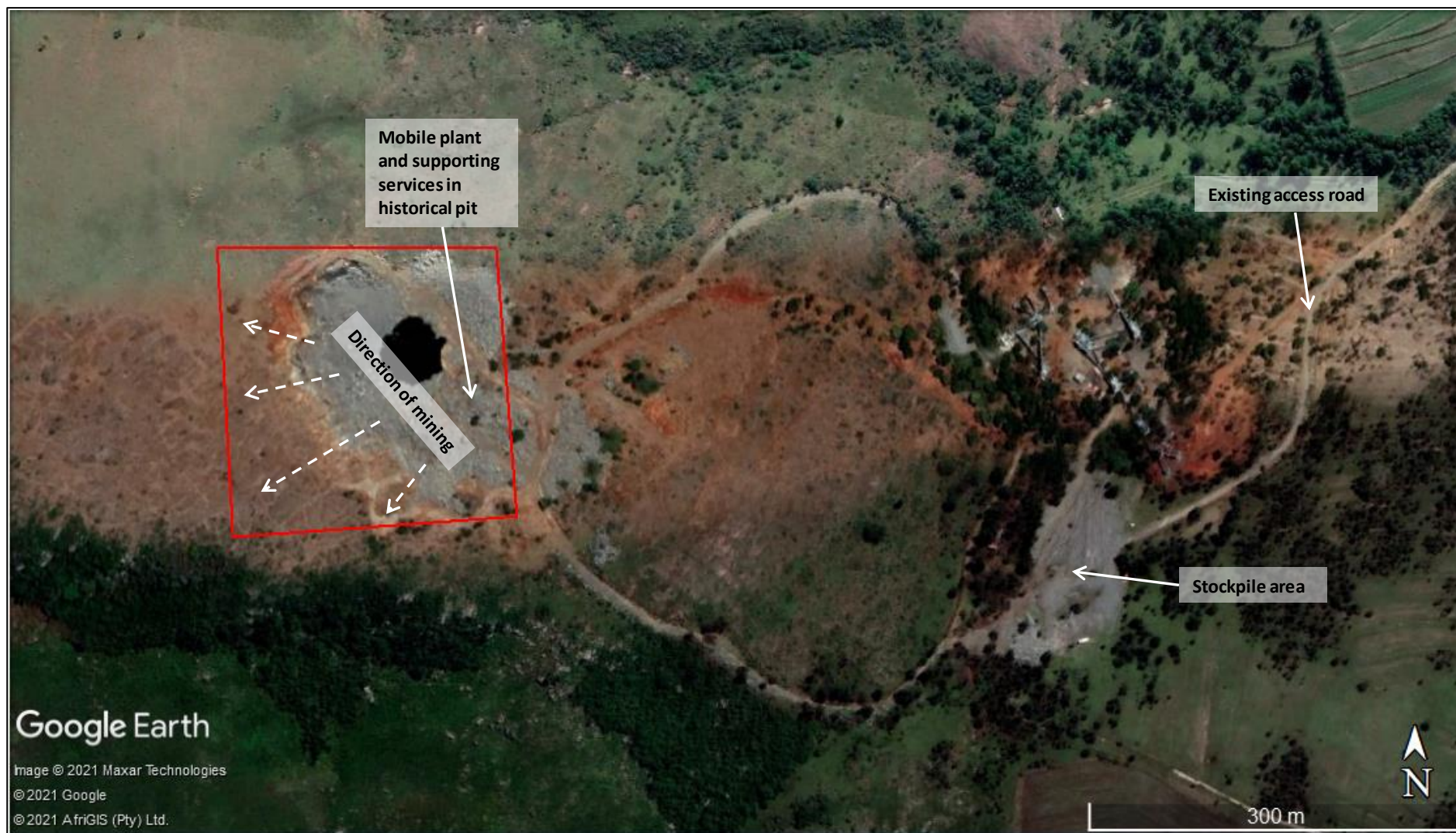
Figure 3: Site layout for the mining operation.
