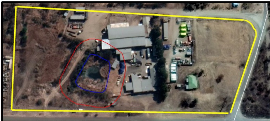
MAP SHOWING THE SENSITIVE SYSTEMS PRESENT WITHIN OR NEAR THE PROJECT SITE (YELLOW POLYGON). THE BLUE AREA INDICATES THE EDGE OF THE QUARRY (WETLAND) AND THE RED LINE INDICATES THE 20M BUFFER ZONE (NO GO AREA).
