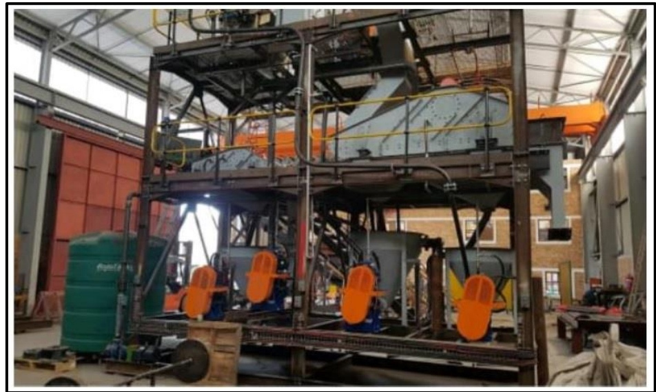
Figure 5: Image showing a typical DMS plant for producing spodumene concentrate (image obtained from Namli Exploration and Mining (Pty) Ltd).
