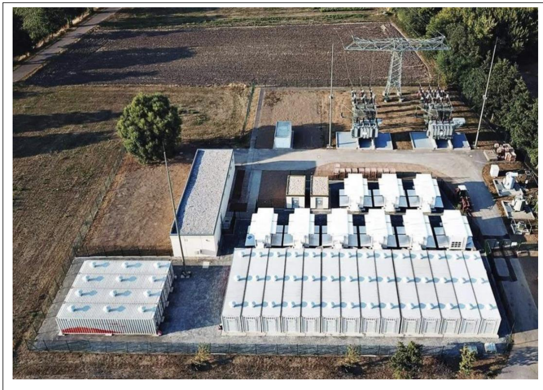
Figure 4: Narada's grid-scale BESS (source: Narada Power Source Co. Ltd, 2018)
