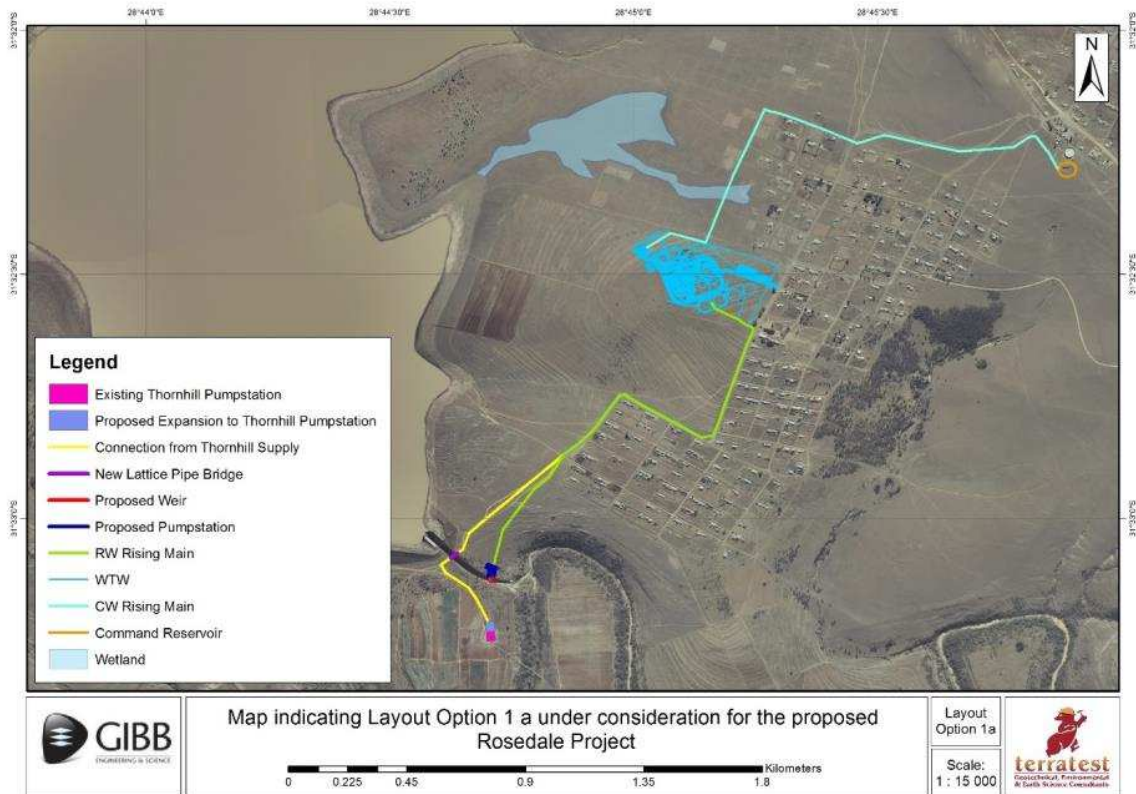
Figure 8: Map indicating the Layout Option 1a for the proposed Rosedale WTW and associated infrastructure.
