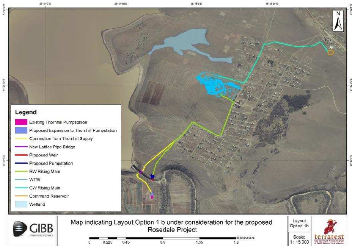
Figure 9: Map indicating Layout Option 1b for the proposed Rosedale WTW and associated infrastructure.
