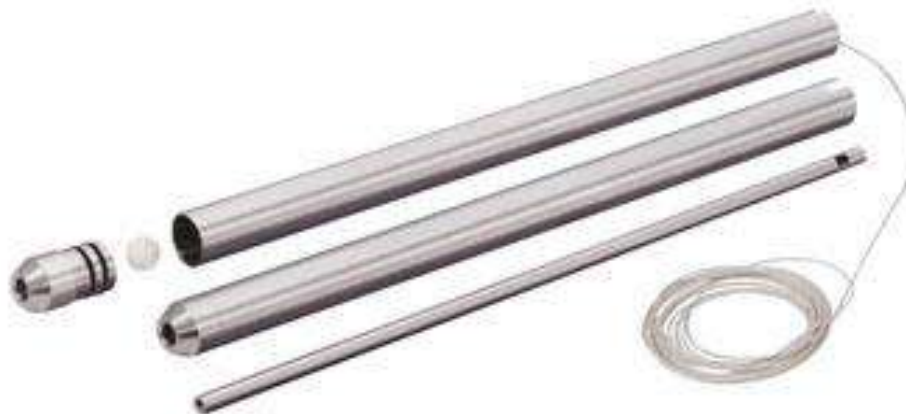
Figure 43: Stainless steel bailer, picture extracted from (Solist, n.d.). A bailer uses a simple ball check valve to seal a sample of the groundwater table at the bottom to raise it up.
