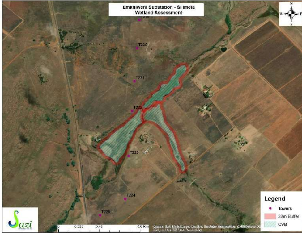
Figure 7: Channelled valley bottom wetland associated with tower 222-225
