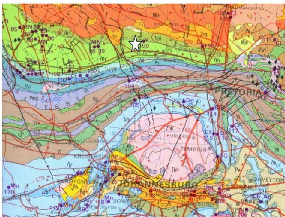
Figure 5.5: Geological Map (Council for Geosciences, 1984) of the region. Star shows site under investigation. Vbi = Bierkraal magnetite gabbro; Vpy = Pyramid gabbro norite.
