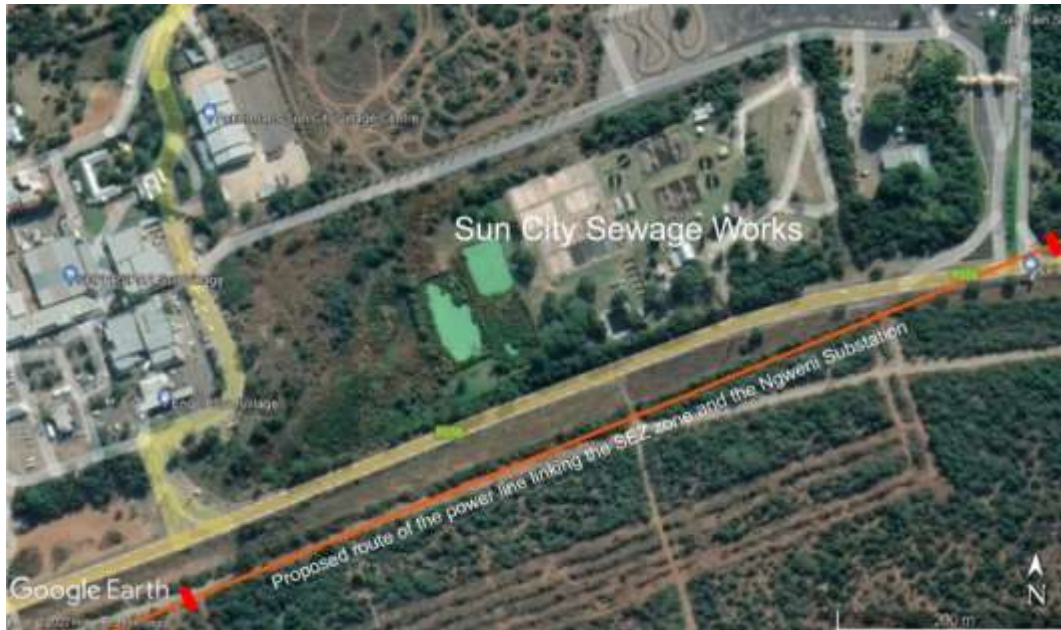
Figure 52. The location of the Sun City sewage works and the proposed power line (orange line) linking the SEZ zone and Ngwedi Substation showing the stretch of line, between the two red markers, that require marking with bird 'flappers'/spirals.
