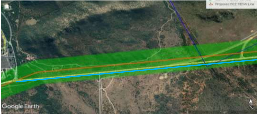
Figure 53. Proposed re-routing of the power line in its western portion showing the positioning of the proposed power line (orange line) north of the R556 road and moved to the south of the road (blue route). The green shading represents a 100 m corridor for power-line. The blue line is the Pilanesberg Nature Reserve/IBA.
