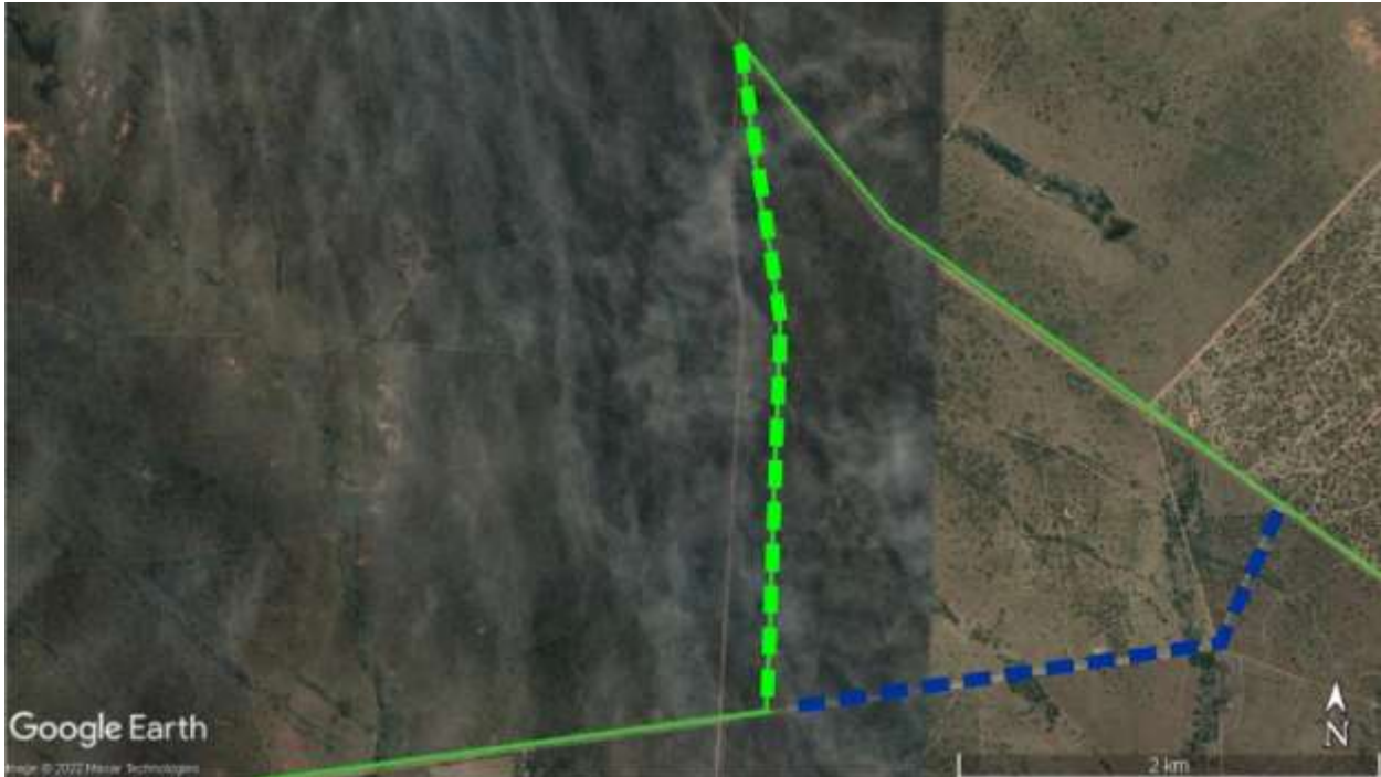
Figure 58: Proposed re-routing of the Bulk WaterLine
