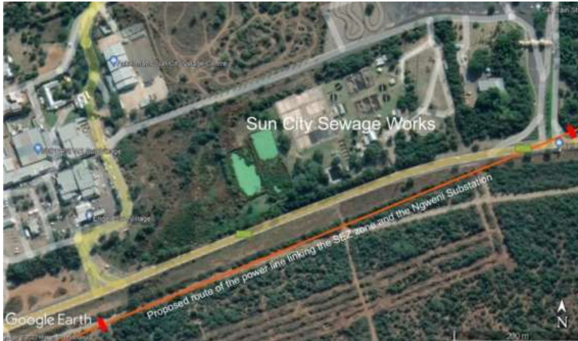
Image 1: The location of the Sun City sewage works and the proposed power line (orange line) linking the SEZ zone and Ngwedi Substation showing the stretch of line, between the two red markers, that require marking with bird 'flappers'/spirals.
