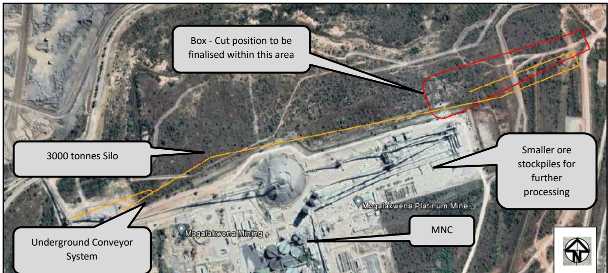
Figure 4-11: Sandsloot Underground Conveyor System Route to M3C 77,78,79,80
