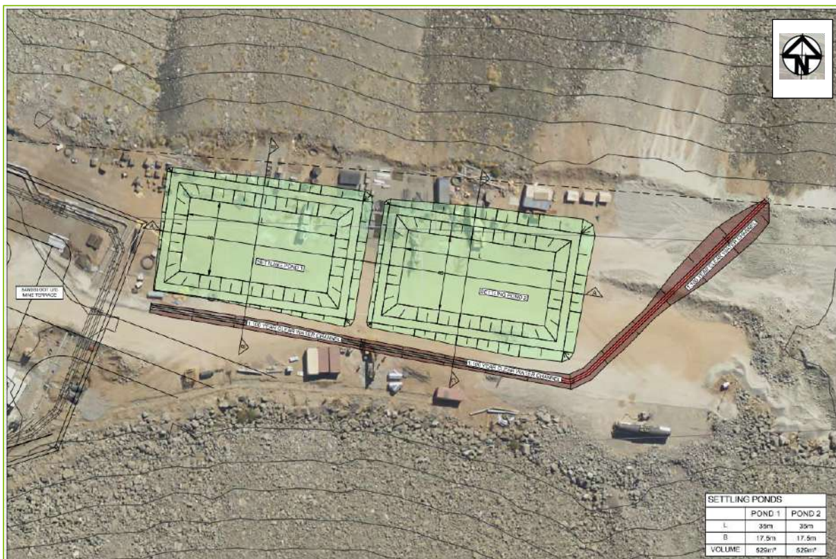
Figure 4-29: Settling Ponds at the Sandsloot Underground Decline Area
