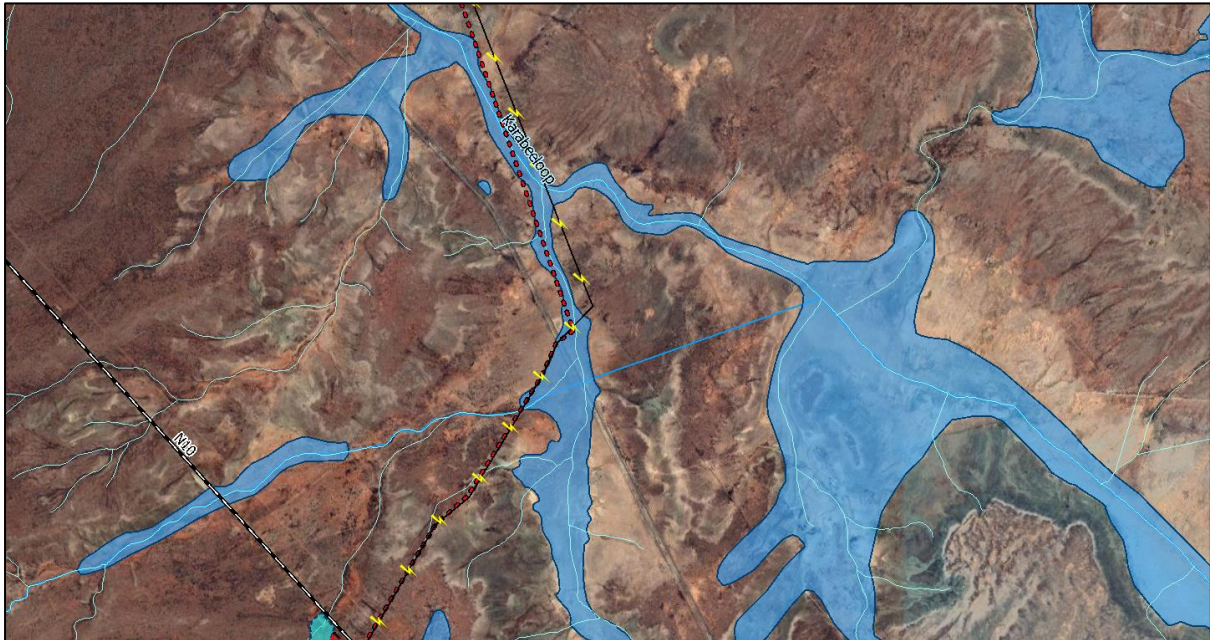
Figure 24 Overview of layout alterations regarding the 132kV transmission line. The new powerline layout (black line with lightning bolts) perpendicularly crosses the Karabeeloo in one location and does not run within the river system as compared to the previous layout (broken red line).
