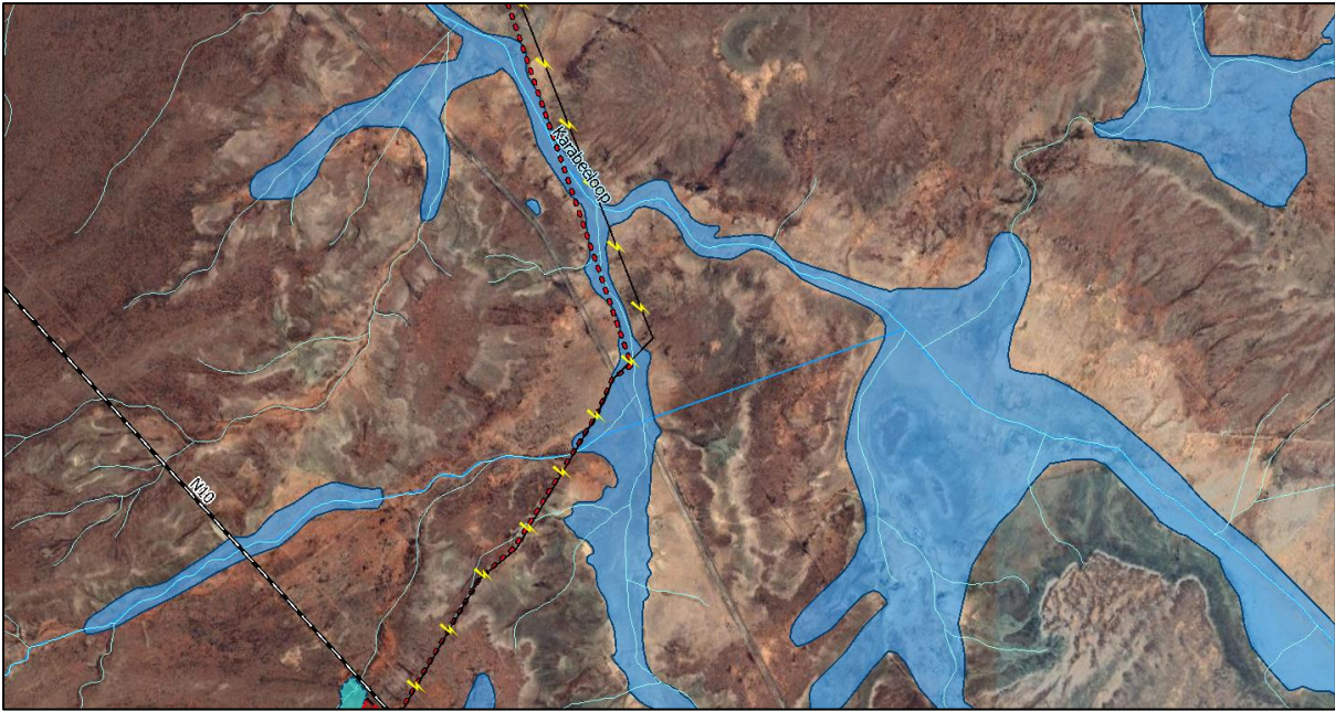
Figure 10 Overview of layout alterations regarding the 132kV transmission line. The new powerline layout (black line with lightning bolts) perpendicularly crosses the Karabeeloo in one location and does not run within the river system as compared to the previous layout (broken red line).
