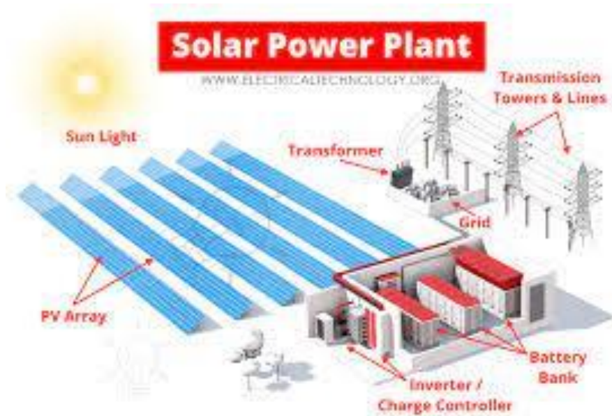
Figure 2.4: Overview of Solar PV Power Plant
