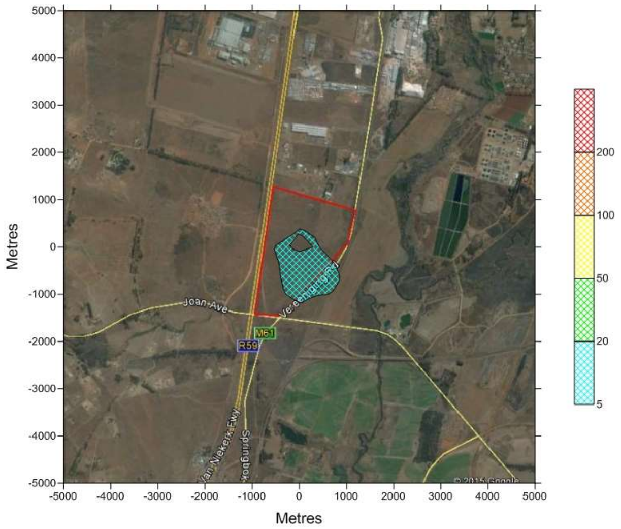
Figure 23. Modeled representation of NO x dispersion from the proposed Waterval PV manufacturing plant. Long term averages, 1 hour averaging period, levels indicated in µg/m 3
