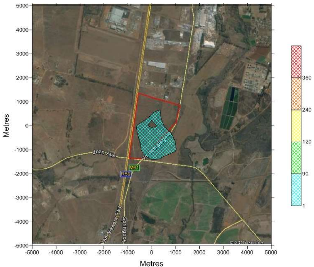
Figure 26. Modeled representation of PM 10 dispersion from the proposed Waterval PV manufacturing plant. Long term averages, 1 hour averaging period, levels indicated in µg/m 3
