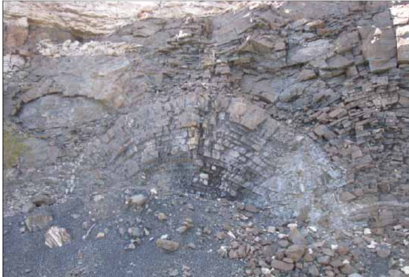
Figure 24: Stromatolites intercepted in pit high walls showing blocky jointing
