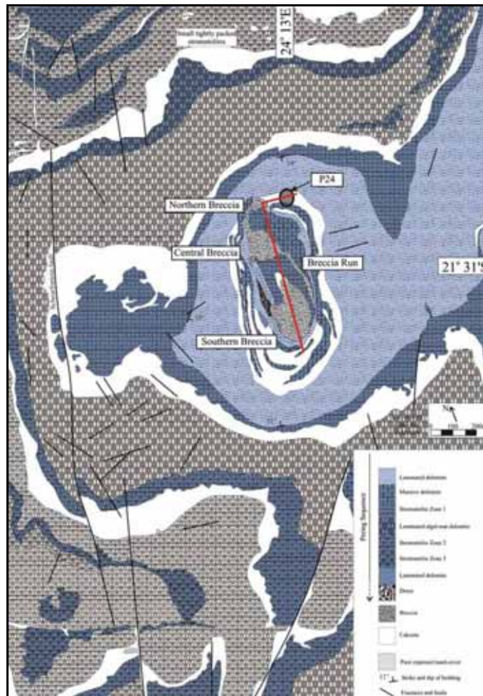
Figure 20: Surface geological map of the Pering deposit and surrounding area (modified after Wheatley et al. 1986)
