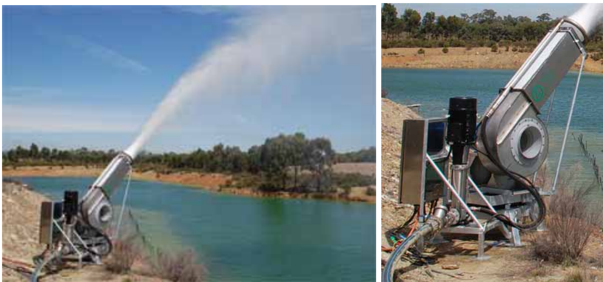
Figure 39: Waste water evaporators ( http://www.wetearth.com.au/Waste-Water-Evaporation )
