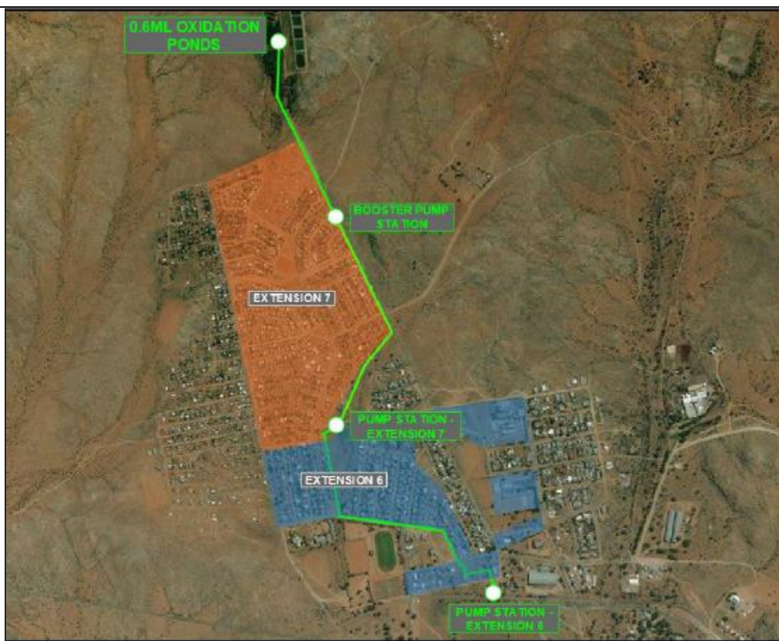
Figure 9. Existing sewage infrastructure servicing the existing Gamakor settlement.
