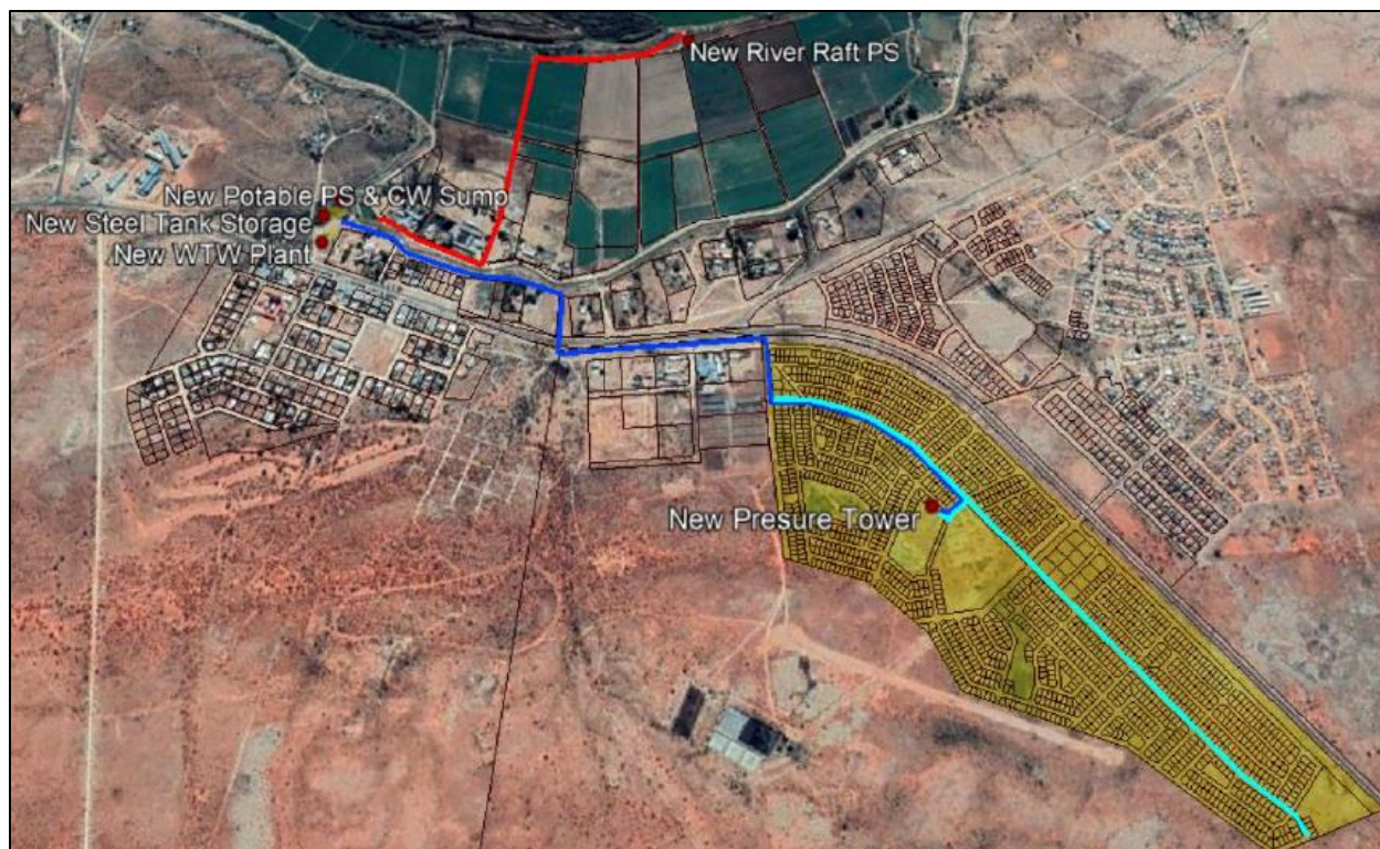
Figure 26. Recommended upgrades to the existing water services for the proposed development of the Groblershoop Housing Project. Source: Engineer's Service Report (Appendix 4B).
