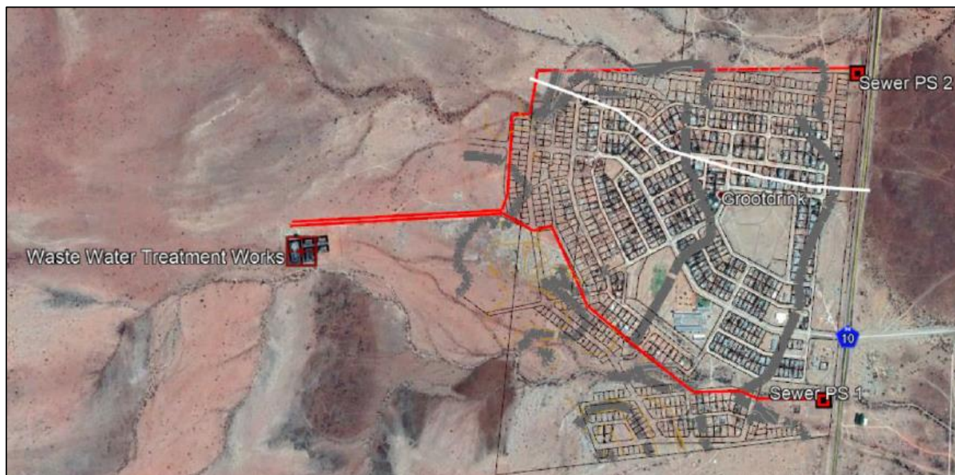
Figure 24. Existing sewage infrastructure servicing the existing Grootdrink Settlement. Source: Engineer's Service Report (Appendix 4B).
