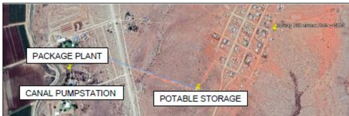
Figure 21. Current water reticulation within the existing Opwag Settlement. Source: Engineer's Service Report (Appendix 4B).
