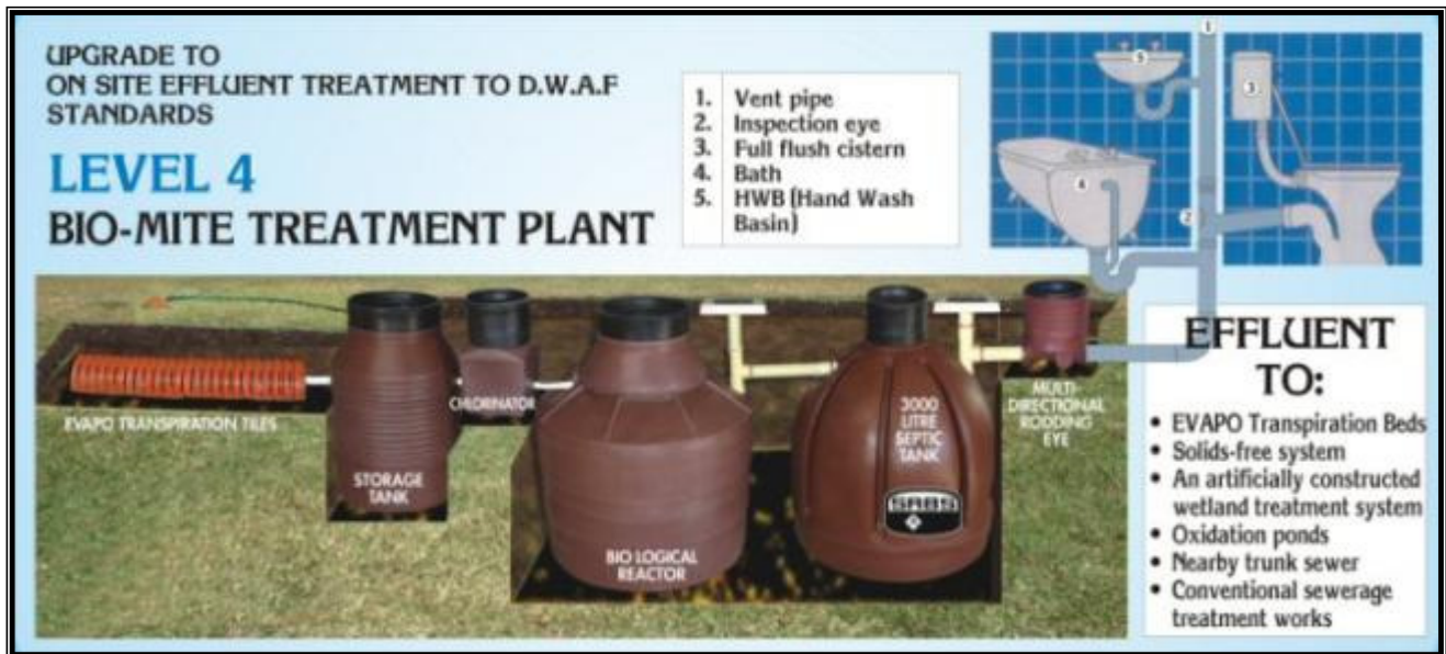
Figure 2.5: Calcamite System at Single Housing Unit (Level 4)
