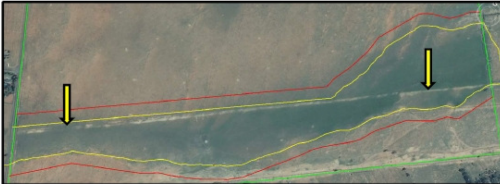
Figure 16: A Close-up of the Drainage Area Downstream of Rooidam. The White Line (Arrows) is a Canal to Contain the Water. The Yellow Line Indicates the Sensitive Wetland Area and the Red Lines Indicate the 50m Buffer Zone to Protect the Wetland from Possible Impacts (Google Earth 2016).
