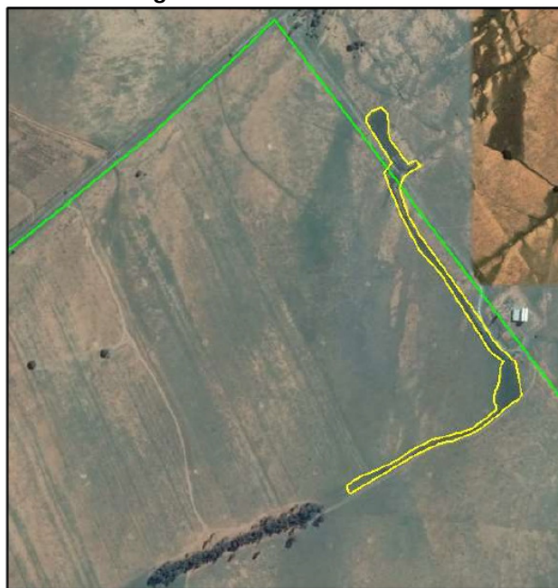
Figure 15: A Close-up of the Wetland which Developed Around a Leaking Water Pipe. The Yellow Line Indicates the Sensitive Wetland (Google Earth 2016). Once the Leak has been Fixed the Wetland will Become Degraded.
