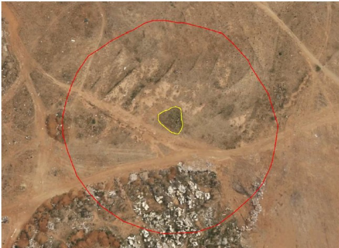
Figure 19: A Close-up of the Depression where Stormwater Collects. The Yellow Line Indicates the Sensitive Wetland Area and the Red Lines Indicate the 32m Buffer Zone to Protect the Wetland from Possible Impacts (Google Earth 2016).
