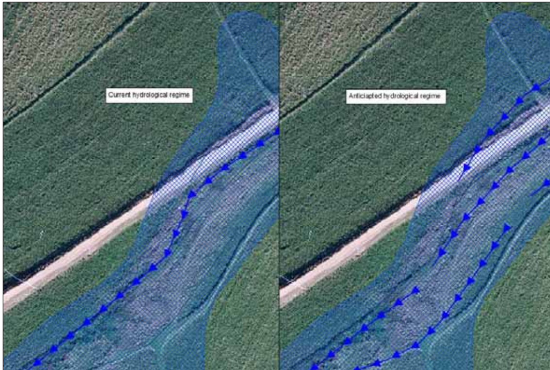
Figure 7-3 An example of the proposed change in hydrological regime following rehabilitation
