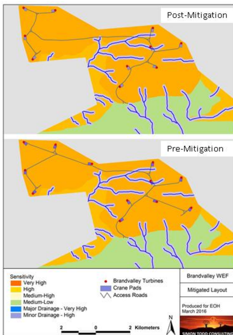
Figure 9-2. Pre and post-mitigation layout of the Snydersberg area, which is considered the most sensitive part of the site. Two turbines have been dropped from the layout and the overall footprint of the development decreased by 39% within the affected area.
