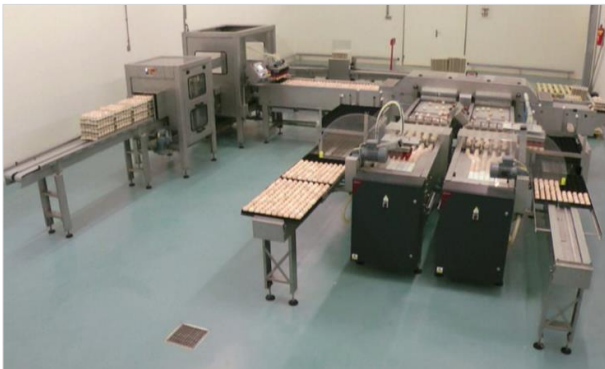
Figure 12: An example of the egg tray to egg setter tray packing machine
