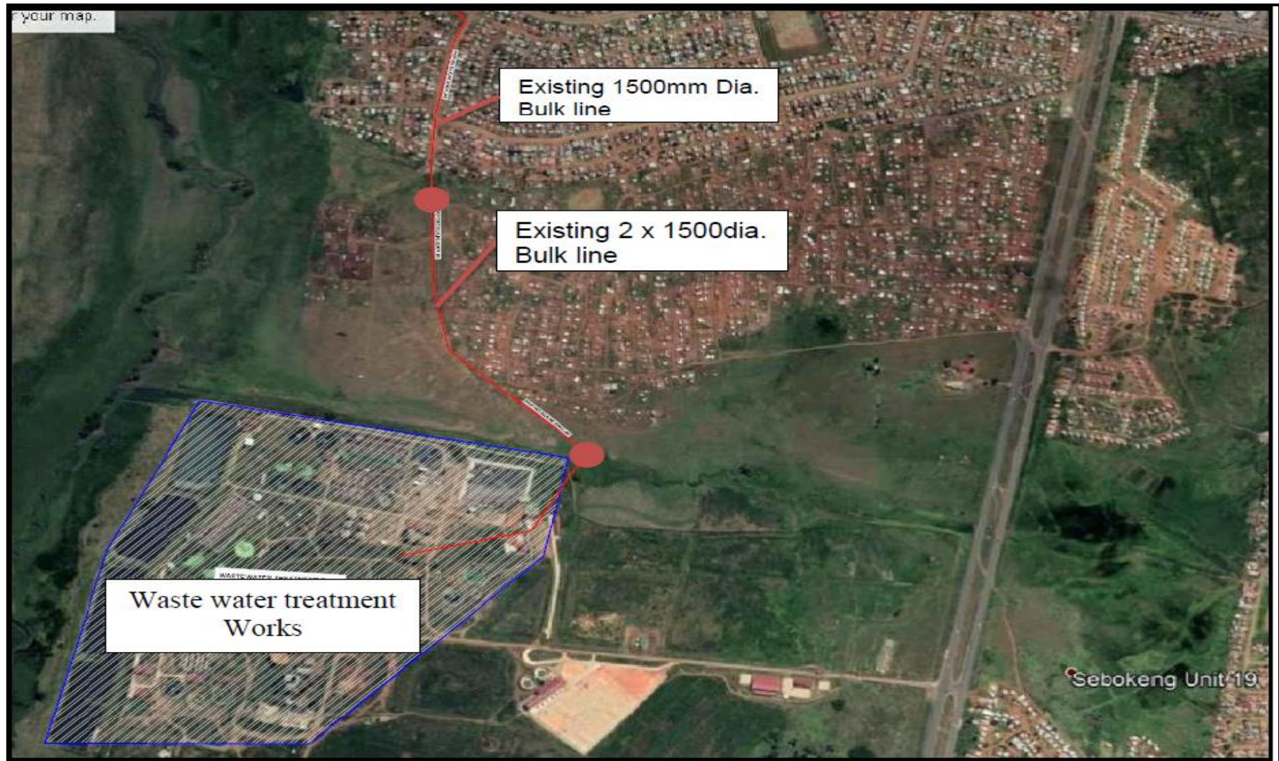
Figure 2: Locality Plan 2-Boitumelo Sewer Pipeline Works
