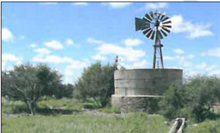
Figure 24: Old wind pump found on Remhoogte, which is still in working condition.
