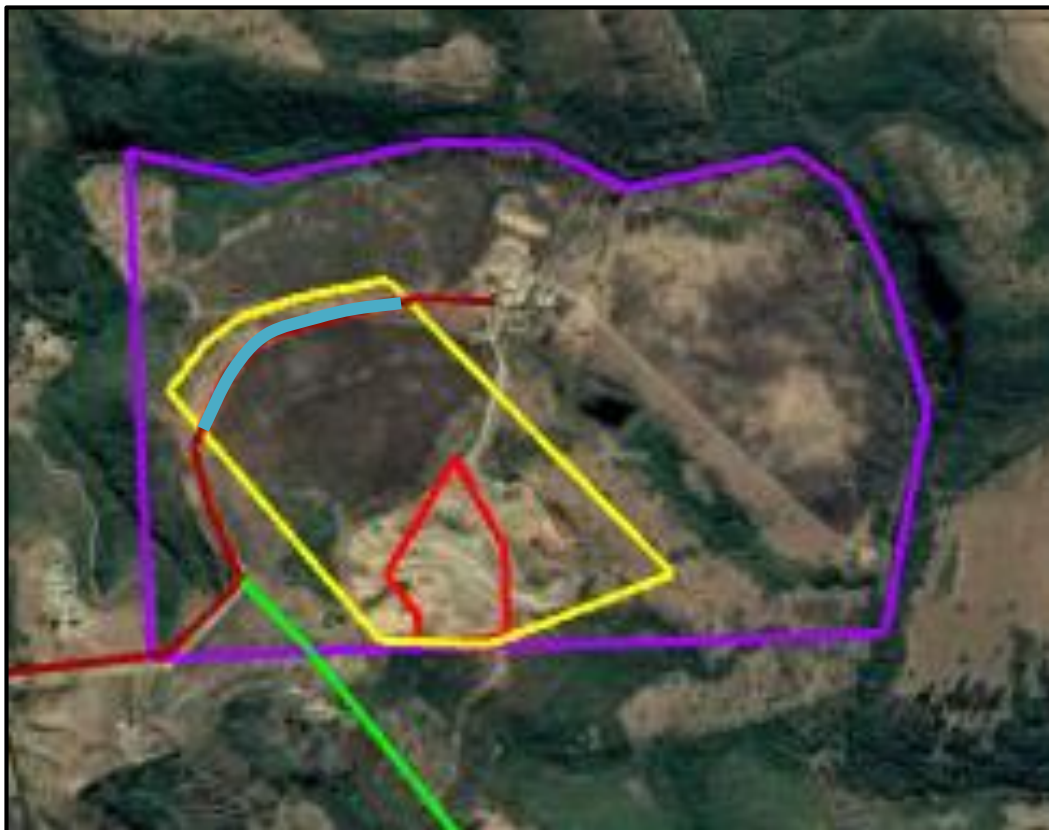
Figure 9: Image showing the section of the W-Road (blue line) that may need re-alignment once mining reaches the most northern part of the footprint area (image obtained from Google Earth).
