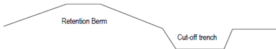
Figure 4: Approximate representation of the recommended berm and cut-off trench system (image obtained from the SWMP).
