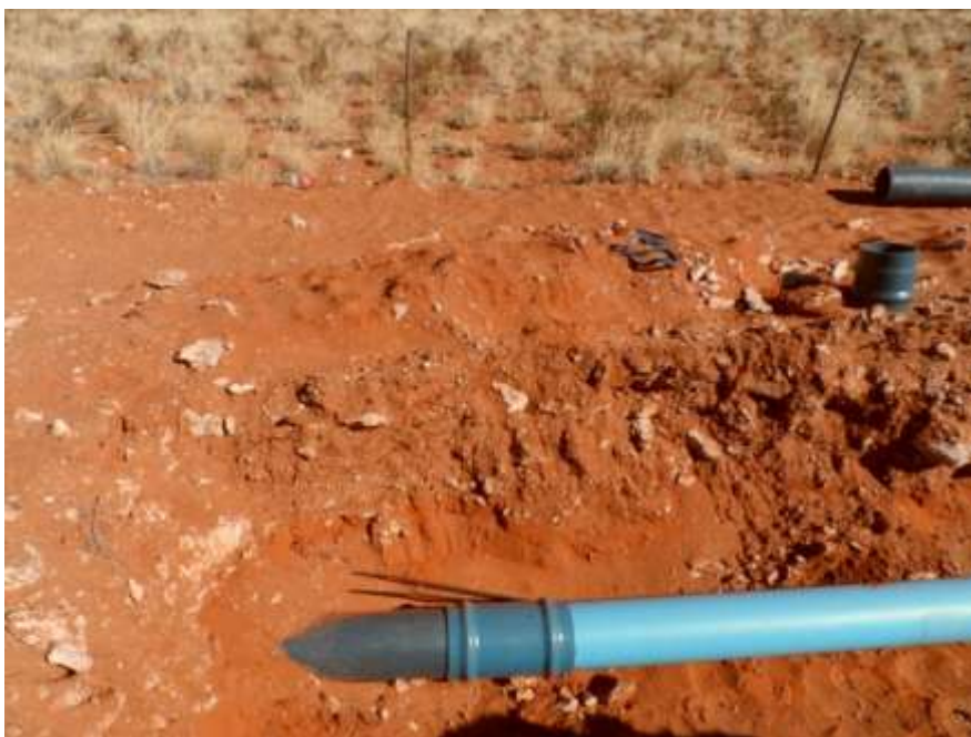
Figure 47: Showing example of the Plooysberg soil form found on the central site alternative (Lubbe, 2013).
