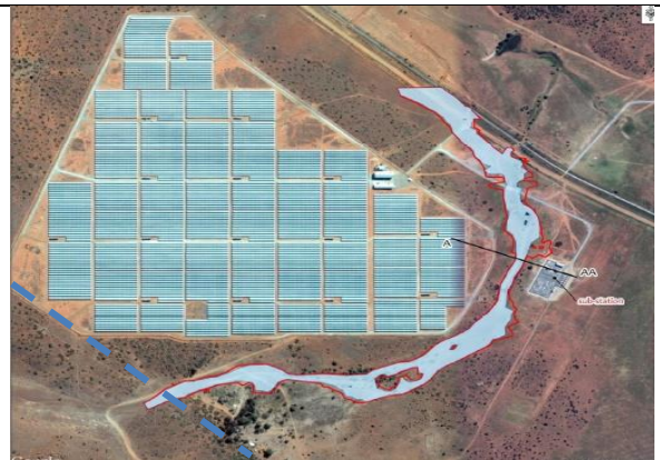
D: Floodline around Lesedi south solar field; blue shaded area shows 1:50-year floodline, and red border shows 1:100-year floodline (Source: Figure 3 of the 2018 Aquatic Assessment and Floodline Determination).
