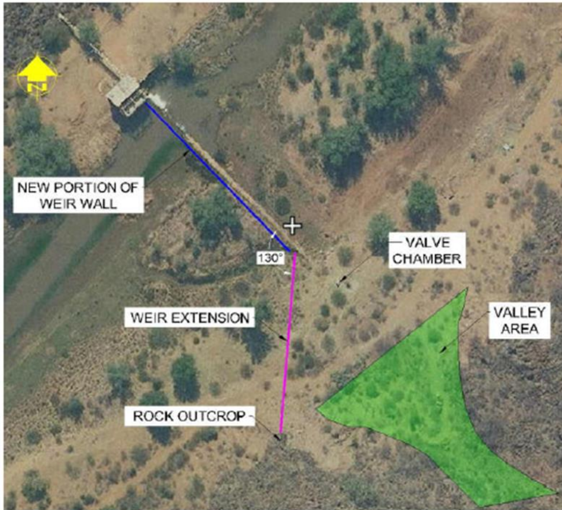
Figure 9: Upgrading of Weir Design
