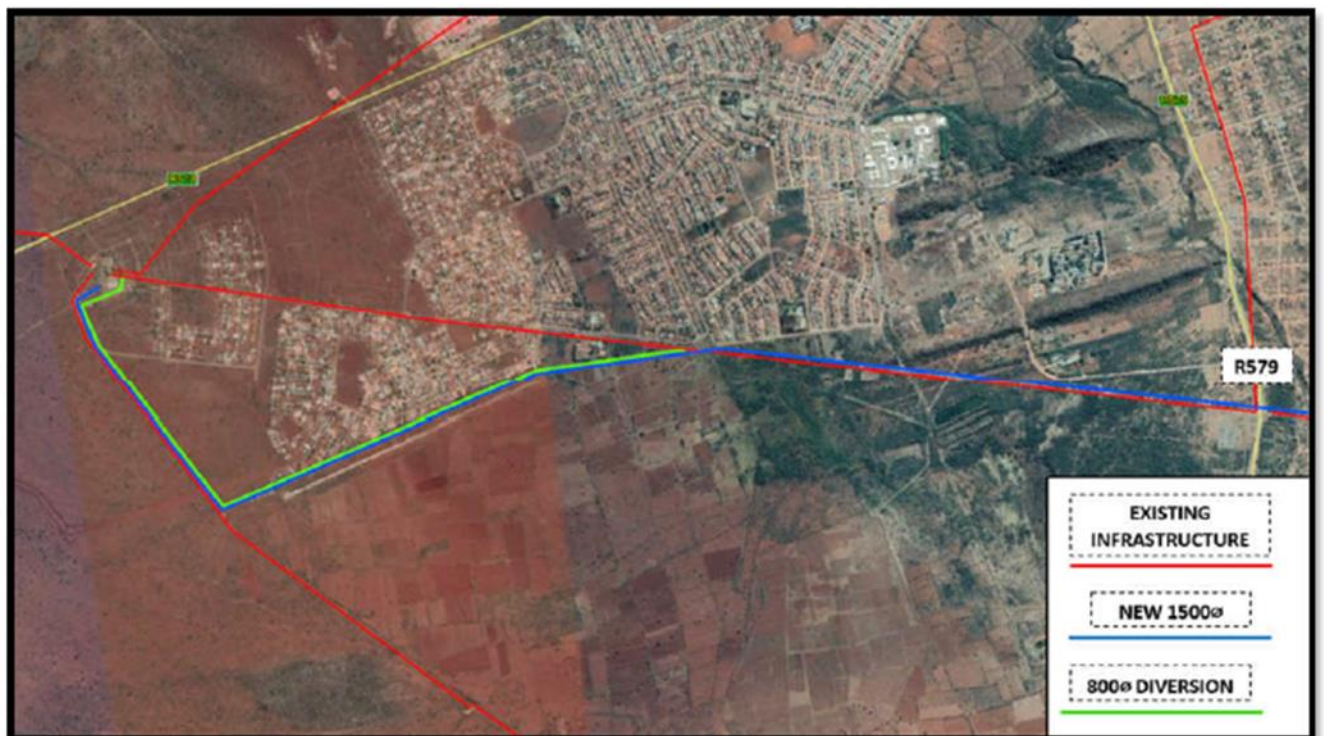
Figure 6: Diversion along Lebowakgomo S (settlements encroached pipeline route)
