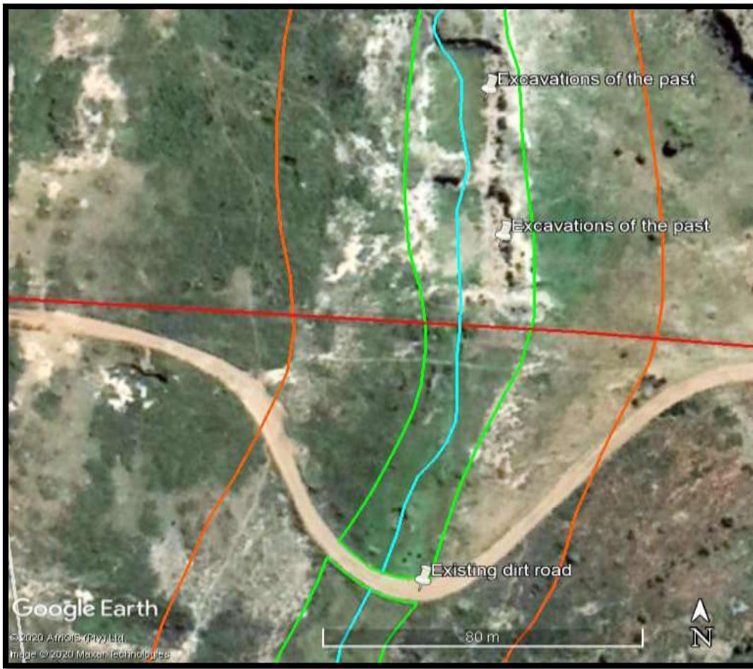
Figure 6: Indication of non-perennial river, riparian zone and buffer zone at the Stream Crossing area at the site.
