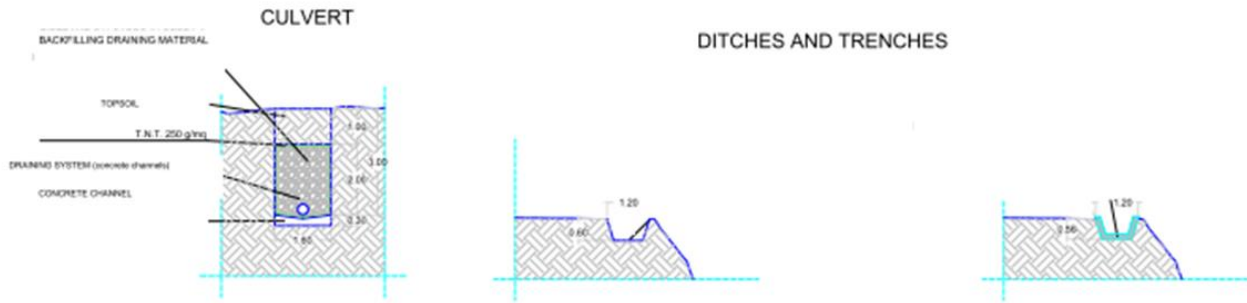
Figure 7-2. Typical culverts and trenches conveying the storm water to the drainage.
