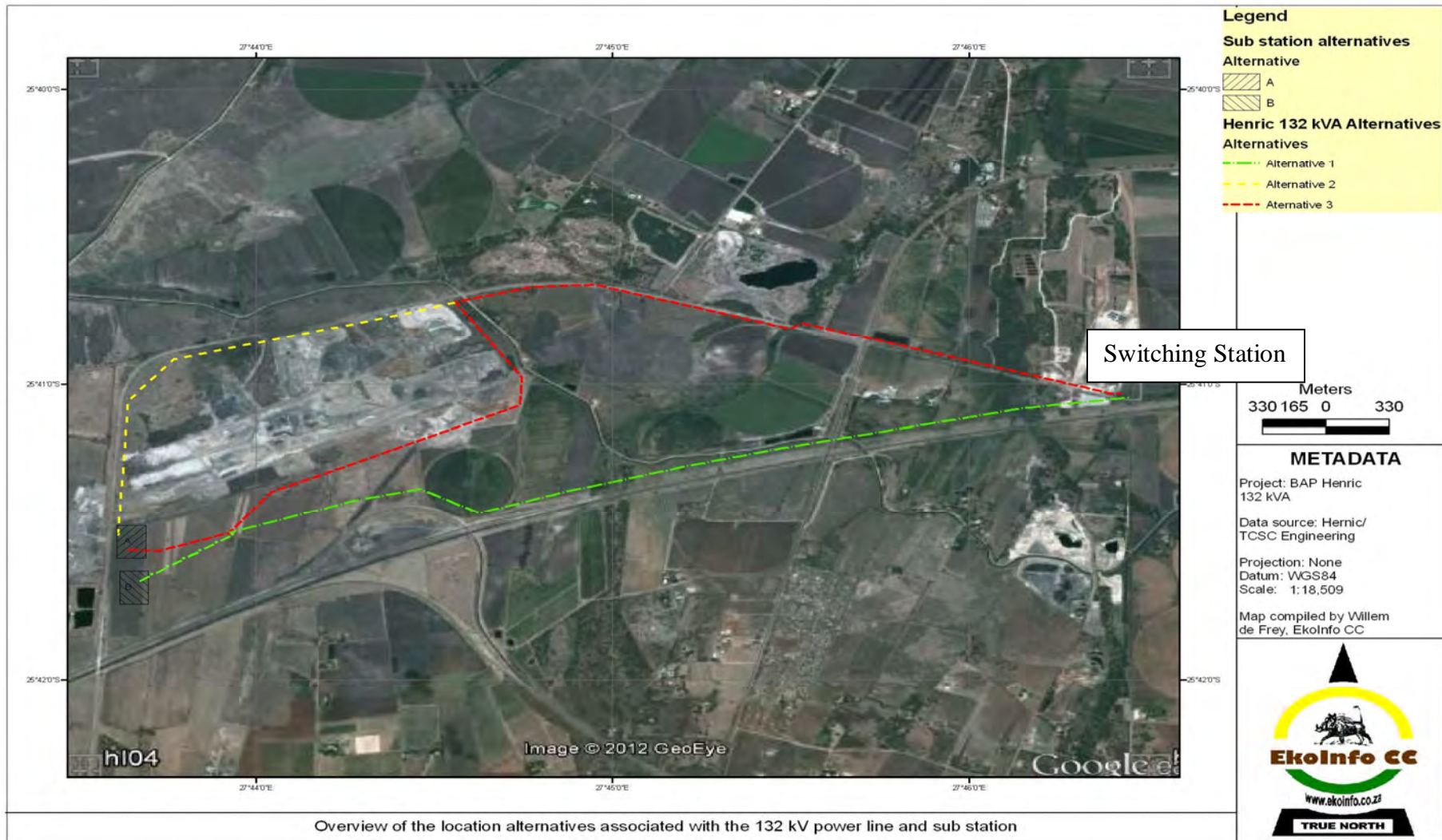
Figure 1 Alternative power line alignment and substation sites
