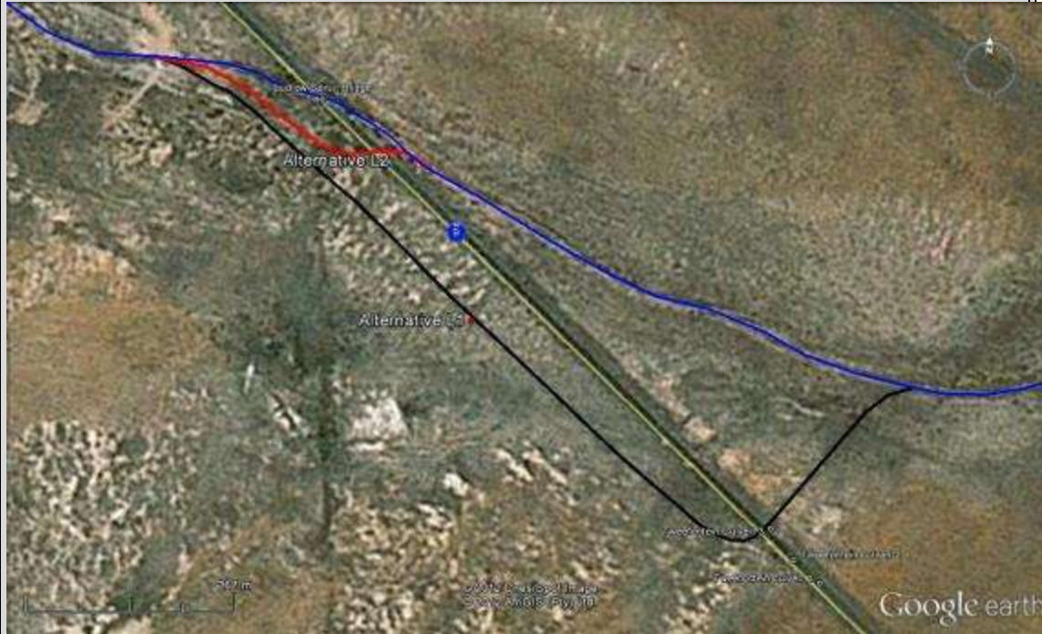
Figure 1: Ludlow Spruit shown in blue with preferred alternative diversion of the spruit (L1) shown in black and alternative L2 shown in red.
