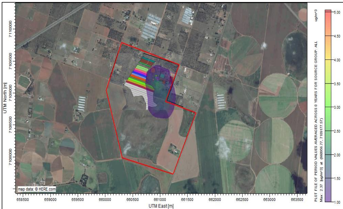
Figure 79: Annual average predicted ambient ground level concentrations ( \mu\text{g}/\text{m}^3 ) of Oxides of Nitrogen (Standard: 40 \mu\text{g}/\text{m}^3 )
