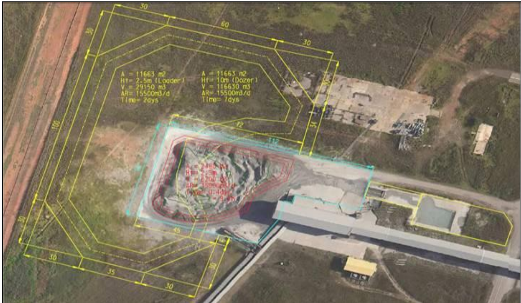
Figure 1-2 - Expansion of emergency dump
