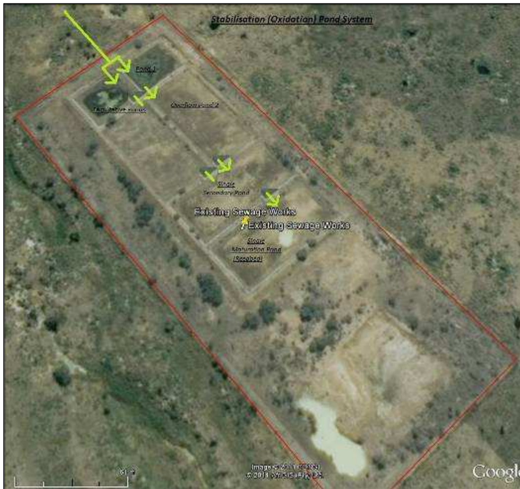
Figure 7: Existing sewerage works flow chart
