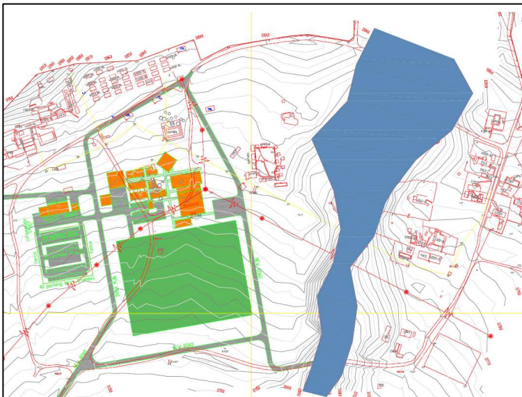
Figure 11: Camp D is affected by a 1:100 year floodline as indicated in blue in this figure. Also refer to Appendix 8 for an A3 drawing indicating floodlines determined for the entire training facility
