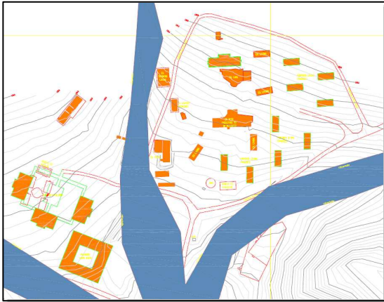
Figure 10: Camp D is affected by a 1:100 year flood line as indicated in blue in this figure. Also refer to Appendix 8 for an A3 drawing indicating flood lines determined for the entire training facility
