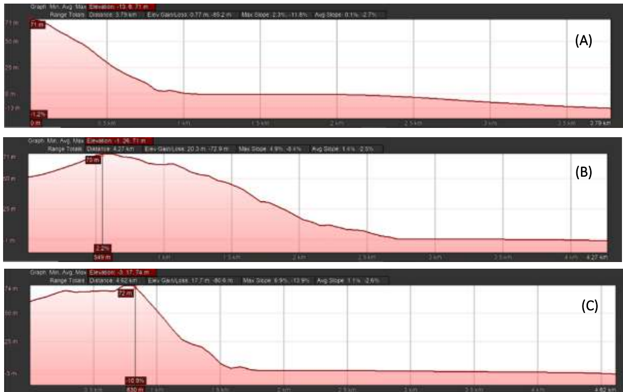
Figure 4.2: Elevation profiles of the proposed development site (a) Inland to the Sea (b) East – West (c) North - South.
