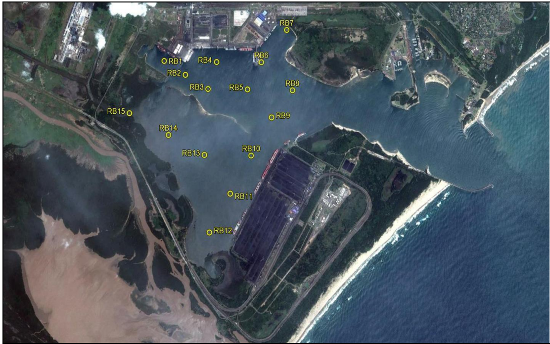
Figure 2-10: Map of Richards Bay showing the positions where in situ water quality measurements were made and water samples were collected for turbidity and total suspended solids concentration analysis in the laboratory
