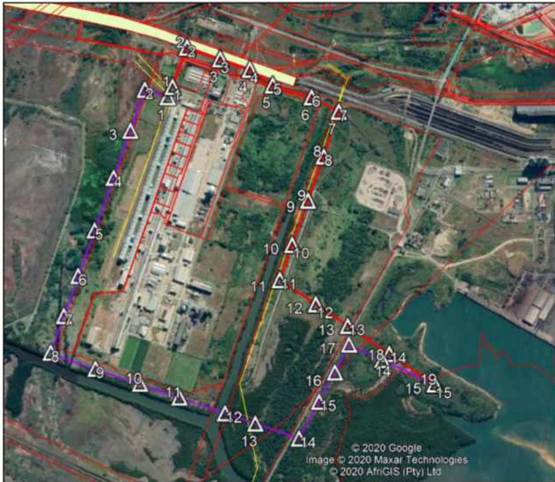
Figure 3-6: Transmission line route alternatives from the Powerships to Bayside substation – Alternative 1 (red) and Alternative 2 (purple). The yellow line is the existing powerline on site.
