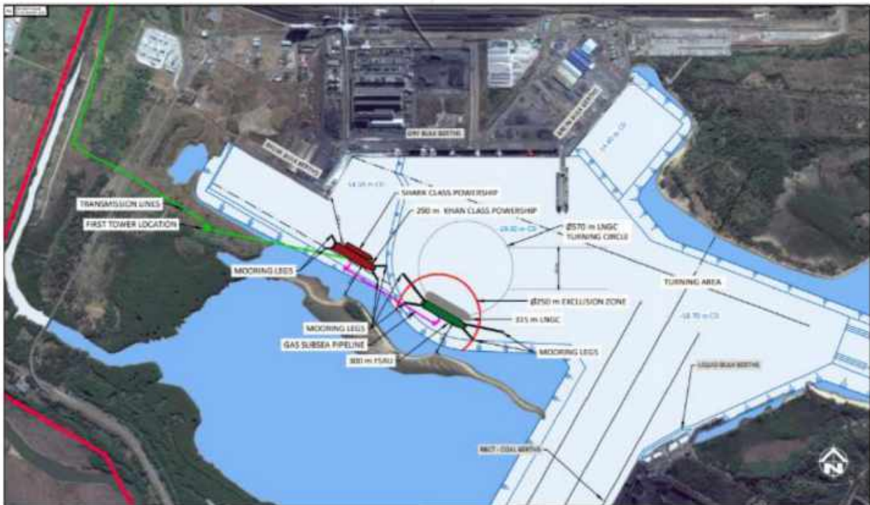
Figure 3-4: Alternative 2: Powership and FSRU position within the port – further from transmission tower
