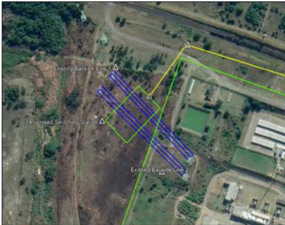
Figure 3-9: Proposed connection to the Eskom line and placement of the switching station
