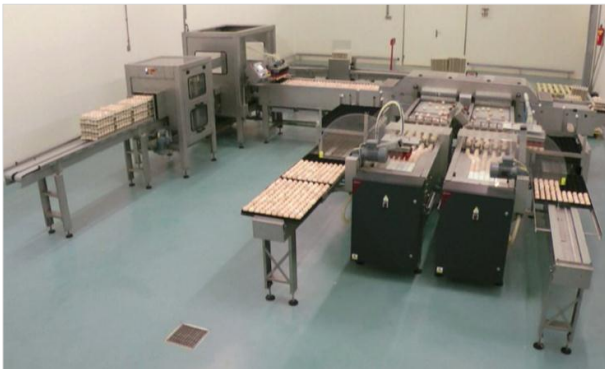
Figure 13: An example of the egg tray to egg setter tray packing machine
