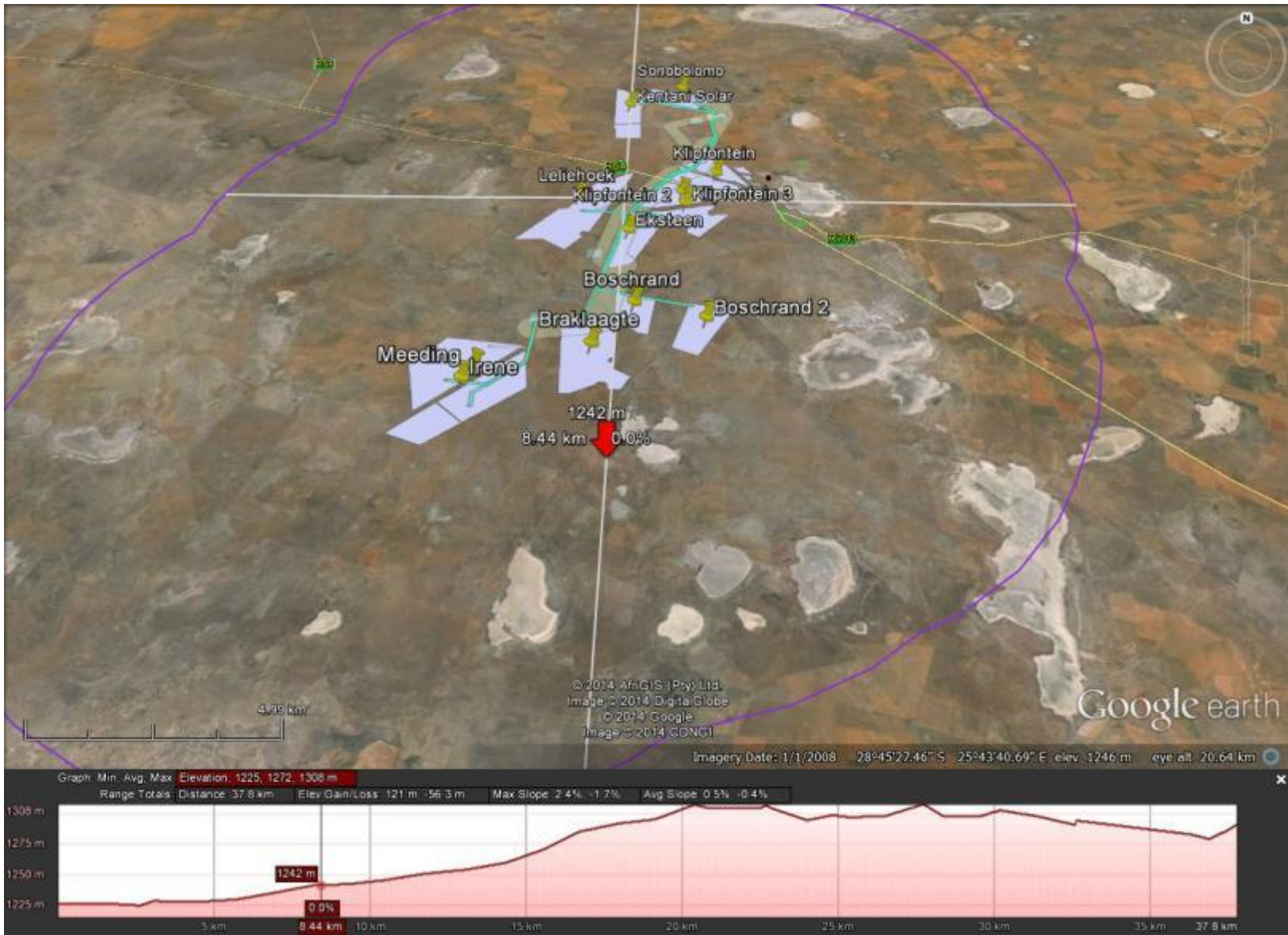
Figure 5.4: Topographic cross-section (grey line) from south to north [within 10 km (purple line)] of the proposed site.
